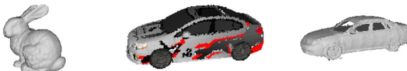
**Fig 9.** Alignment results of three individual scan batches: Stanford bunny (left), WRX (center), and the Legacy dataset (right). Through the use of the painting-assisted alignment, highly symmetrical scans can be effectively aligned with minimal human intervention.
