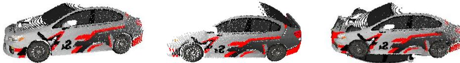
**Fig 6.** SAC-IA fails to provide an accurate alignment (right) of the two input point-clouds (left and center) due to the influence of the incorrect correspondence between the trunk and hood.
